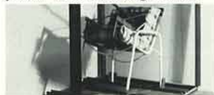
Rack 'n Roll Machine: torture test for legs.
