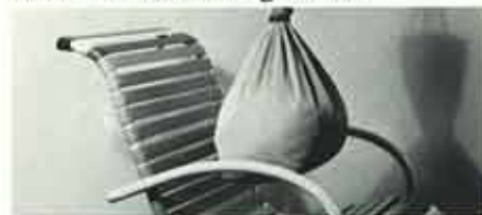
Sock-It-To-Me-Test: a 620-pound punch—but no buckling allowed.
